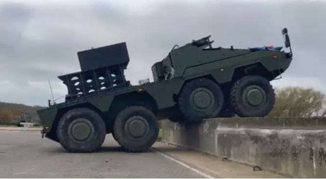
Boxer DM with representative RCH155 weight and CofG climbs a 1m step... @ UK MOD
