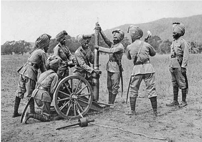
Figure 2. 2.5 inch Gun Drill. Separating the barrel into its two parts © Wikipedia.
